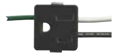
*22532 Snap-in Outlet with Ground Wire Black 6" Wire Leads 14 Gauge 15A, 125 Volts Fits 1" Square Opening with Green Ground Wire Height - 7/8"
