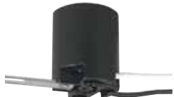
*22215 1 ½" Socket 6" Wire Leads and Straight Bracket Medium Base 18 Gauge, 105° Leads Bracket Extends 1½" Measured Center to Center 660 Watts Max., 250 Volts Height - 1½"
