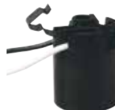
*22217 1 ½" Snap-in Socket 9" Wire Leads Medium Base Fits ¾" x ¼" Hole 18 Gauge 105° Leads 660 Watts Max., 250 Volts Height - 1½"
