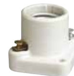
*22273 Porcelain 1-Piece Receptacle Medium Base 660 Watts Max., 600 Volts Height - 1½" 180° C Maximum Temp.
