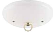
70037 Modern Canopy Kit with Center Hole White Finish 5" Diameter, 7/16" Center Hole 40 lb. Load Rating Includes: 1 Canopy, 1 Screw Collar Loop, 2 Mounting Screws, 1 Lock Washer, 1 Locknut
