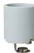
*22267 Porcelain Keyless Socket Medium Base ½-IP Hickey 660 Watts Max. 250 Volts Height - 2" 1875 Pulse Rated
