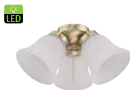
77845 LED Cluster Ceiling Fan Light Kit Polished Brass Finish Frosted Ribbed Glass Diameter: 12.75" Height: 7.00" Includes (3) Medium (E26) Base, 5 Watt Omni A15 LED Lamps
