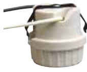
*22212 Porcelain Snap-In Socket Medium Base 6" Wire Leads Fits 1½" Hole 18 Gauge, 125° Leads 660 Watts Max., 250 Volts Height - 1¾"
