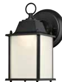
61075 Dimmable LED Wall Fixture Textured Black Finish Frosted Glass Height: 8.50" Width: 4.50" Extends: 6.00" Height from Center of Outlet Box: 2.63" Back Plate: D: 4.53" Includes 9 Watt Integrated LED
