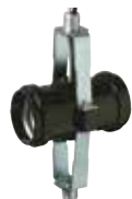
*22259 Twin Cluster Socket with Male Threads on Each End Medium Base 6" Wire Leads, 18 Gauge 105° Leads 660 Watts Max., 250 Volts ½-IP Nipple Height - 4¾"
